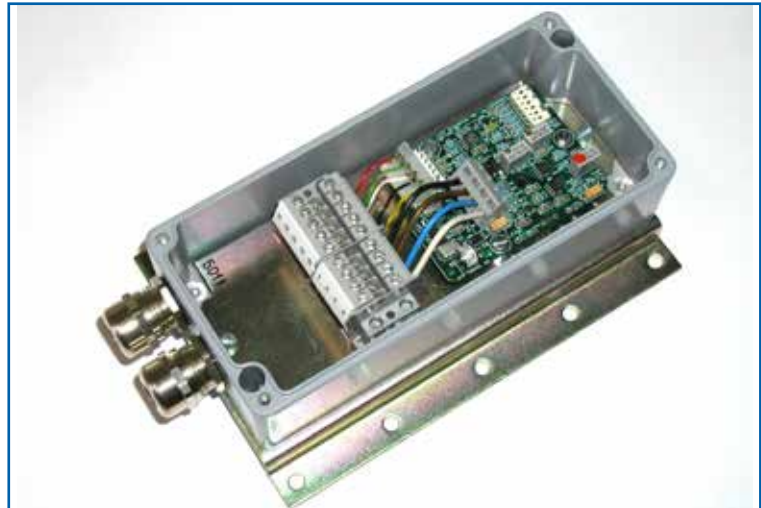
Top view of the PIAB LCA Load Cell Amplifier without top cover. It gives an output signal of 4-20mA.
