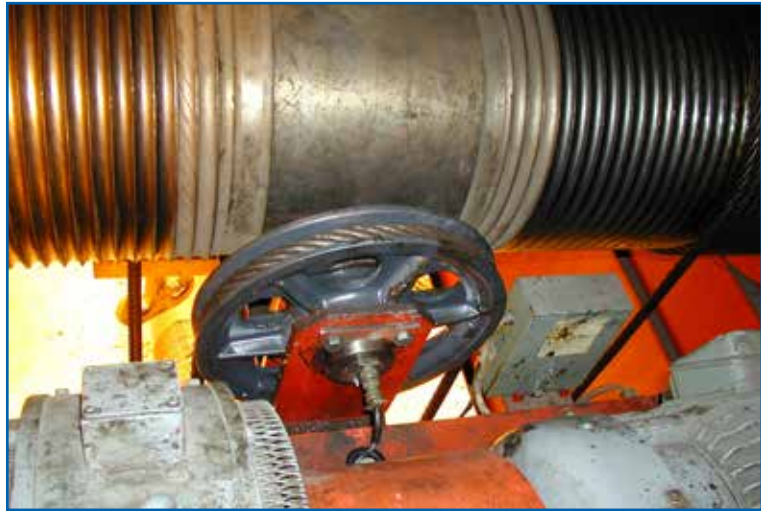
PIAB Load Pin SLC mounted in an equalisation sheave.
