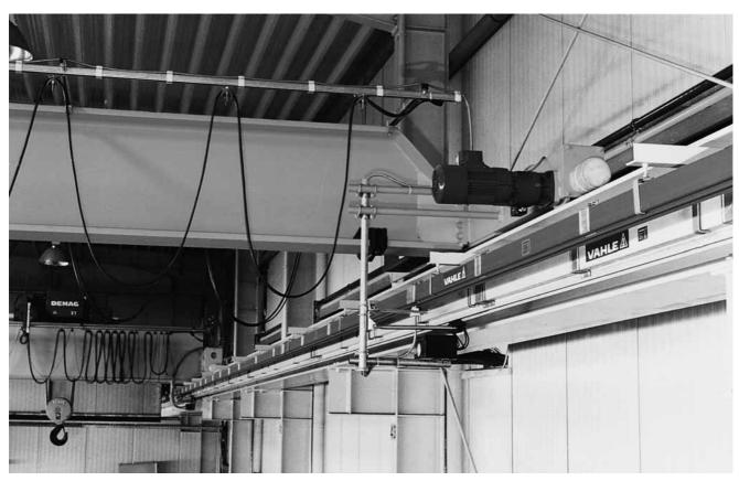
Powerail for the current supply of a hangar crane.
